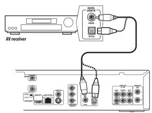
**Optical connection:** Use an optical cable (not supplied) to connect the **DIGITAL AUDIO OUT – OPTICAL** jack to an optical input on your AV receiver.
